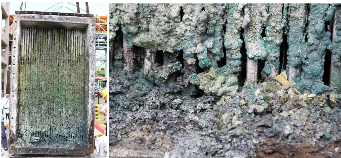
Figure 6. Evidence of Fouling due to insufficient ammonia destruction in a thermal oxidizer
