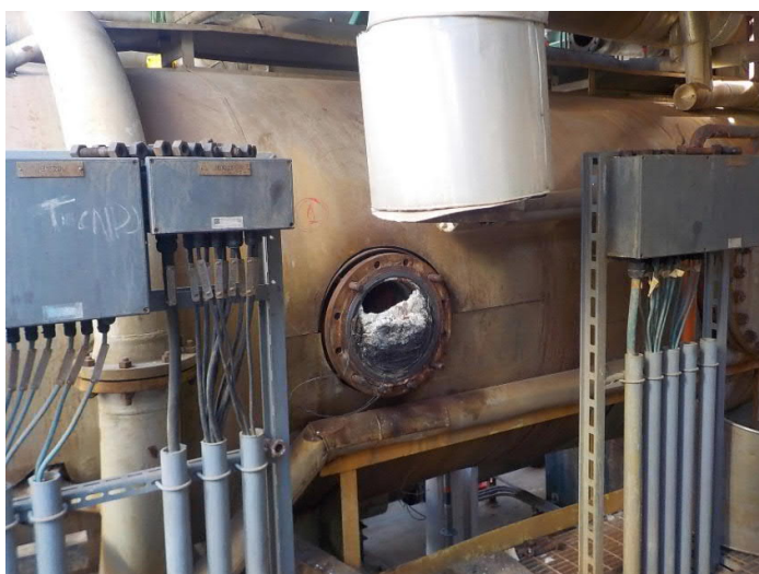
Figure 3. Evidence of ammonium salt plugging on incinerator nozzle
